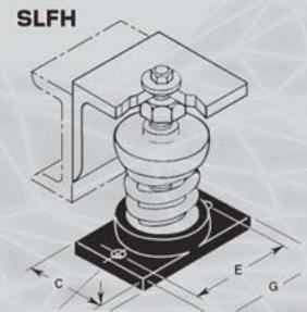
C housed spring mounts are more economical choice for outdoor applications. They have lateral stability and are recommended for moderate horizontal wind loads without seismic restraint requirements.
